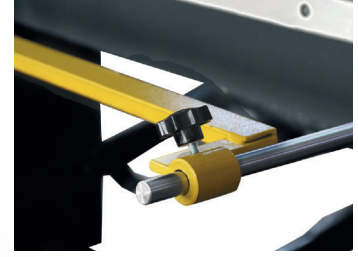
Kolay ayarlanabilen arka dayama Back gauge with easy setting
