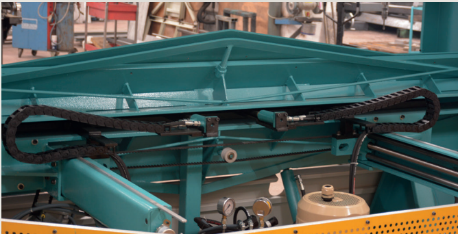
·1 Otomatik + 1 Eksen Manuel ayarlanan Arka Dayamalar ·1 Automatic + 1 Axis Manual Adjustable Backgauge 1000mm
